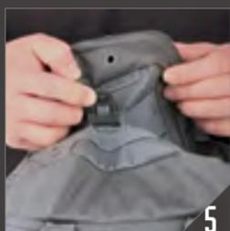
5 Insert the tail under the bridge, making sure both the tab and the tooth have both clicked into place.
