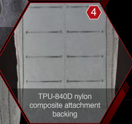
TPU-840D nylon composite attachment backing
